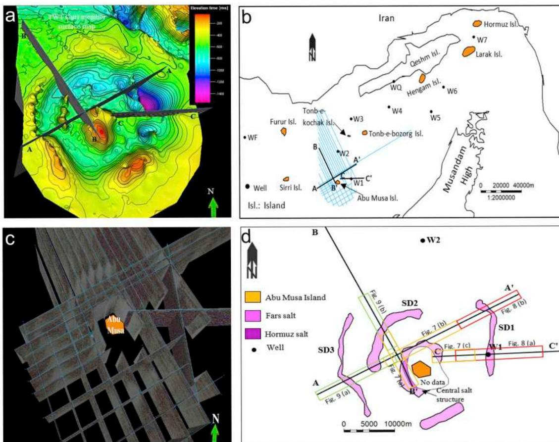
**Fig. 3.** (a) Guri member structure map of the Abu Musa diapir (b) the location of AA', BB' and CC' seismic sections along the NE-SW, NW-SE and E-W trends, respectively. (c) Sketch map of the Abu Musa Island on the seismic sections (d) Sketch showing the location of Abu Musa Island and identified buried salt structures within the Abu Musa diapir as the Fars salt structures.
