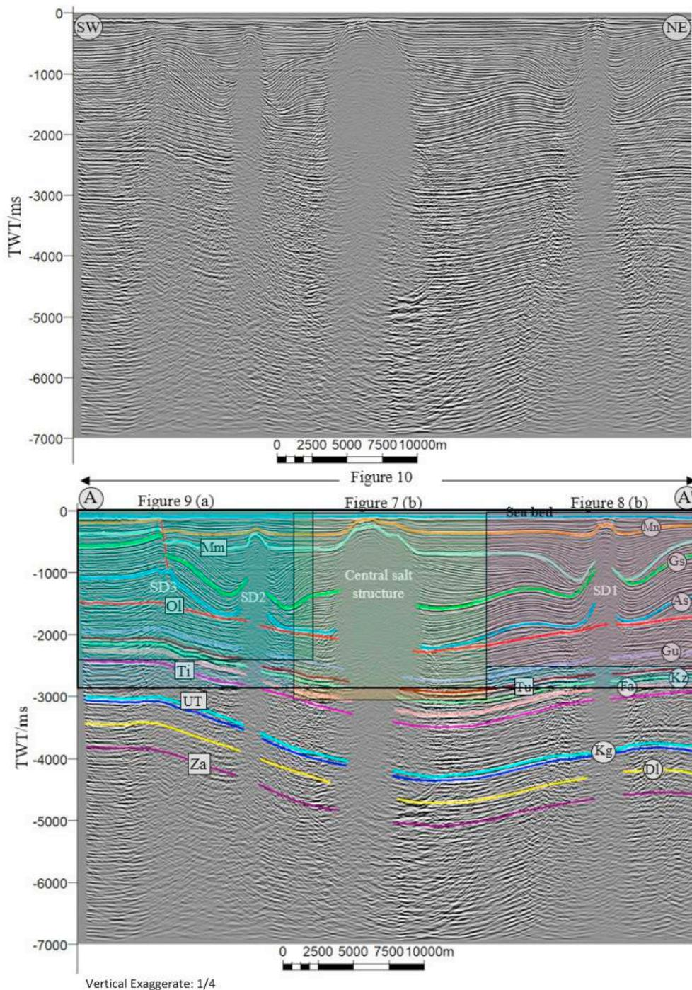
Fig. 4. Un-interpreted and interpreted AA' seismic sections NE-SW through the Abu Musa salt diapir. The interpreted SD1, SD2, SD3, the upper part of central salt structures, the location of seismic horizons (letters in circles) and major unconformities (letters in rectangles) are presented. Abbreviations as per Fig. 2 caption. Location of Figs. 7–10 shown by rectangles.
