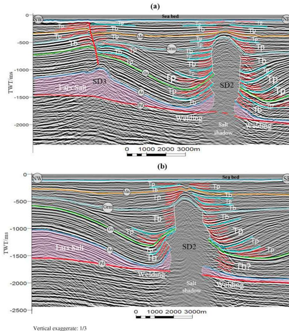
**Fig. 9.** (a, b) Un-interpreted and interpreted seismic sections showing halokinetic sequences on the SD2 and the SD3 salt structures along AA' and BB' (locations as per Figs. 4 and 5). "Tb" and "Tp" connote the tabular and tapered halokinetic sequences, respectively. Details of the used letters in Fig. 2.
