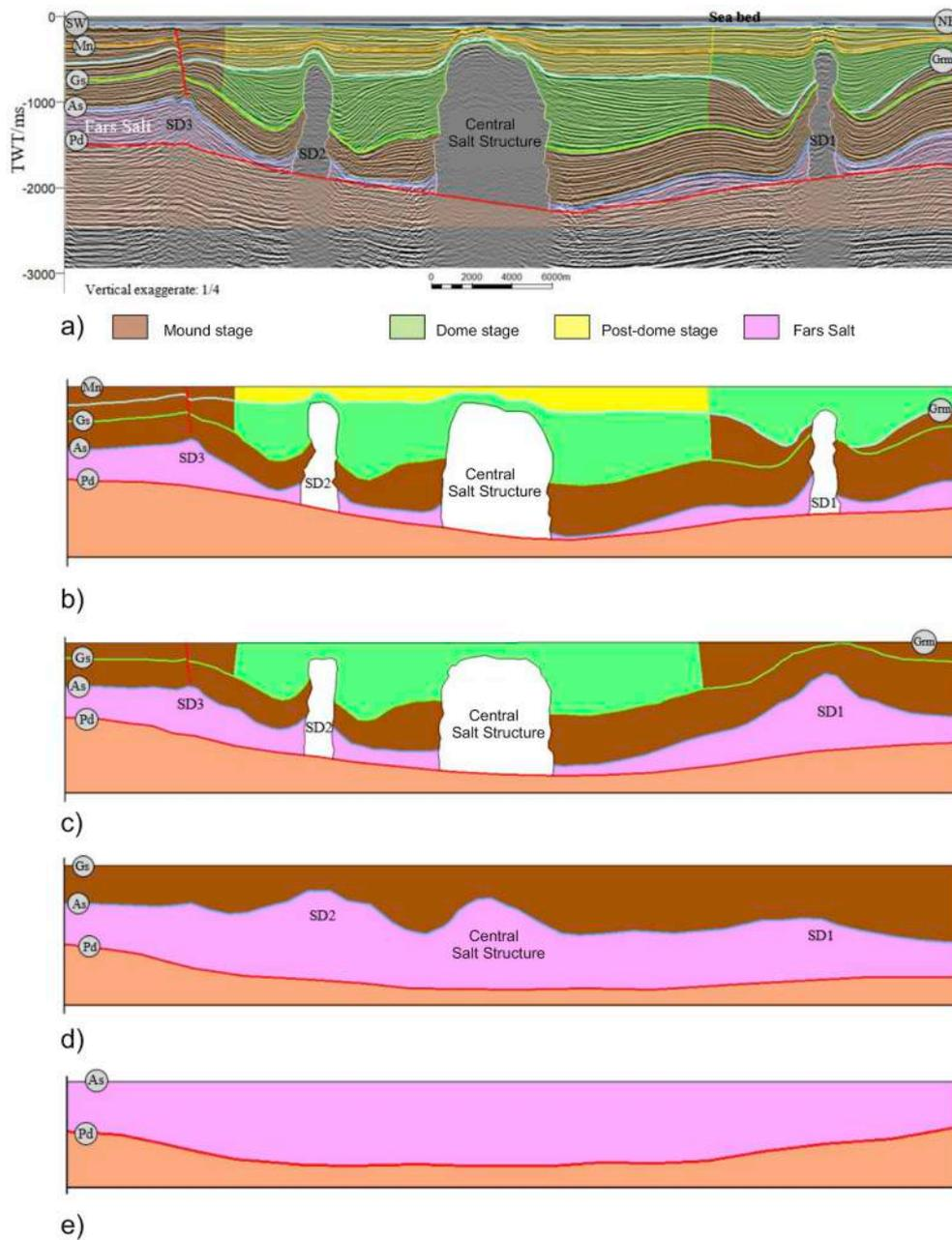
**Fig. 10.** Schematic evolutionary stages of the Central, SD1, SD2 and SD3 salt structures in the Abu Musa salt diapir. The sections obtained based on the method introduced by Gilardet et al., 2013). a) present-day configuration of the salt structures. b) Flattened section on the Mishan horizon. c) Flattened section on the Guri member horizon. d) Flattened section on the Gachsaran horizon. e) Flattened section on the Asmari horizon.
