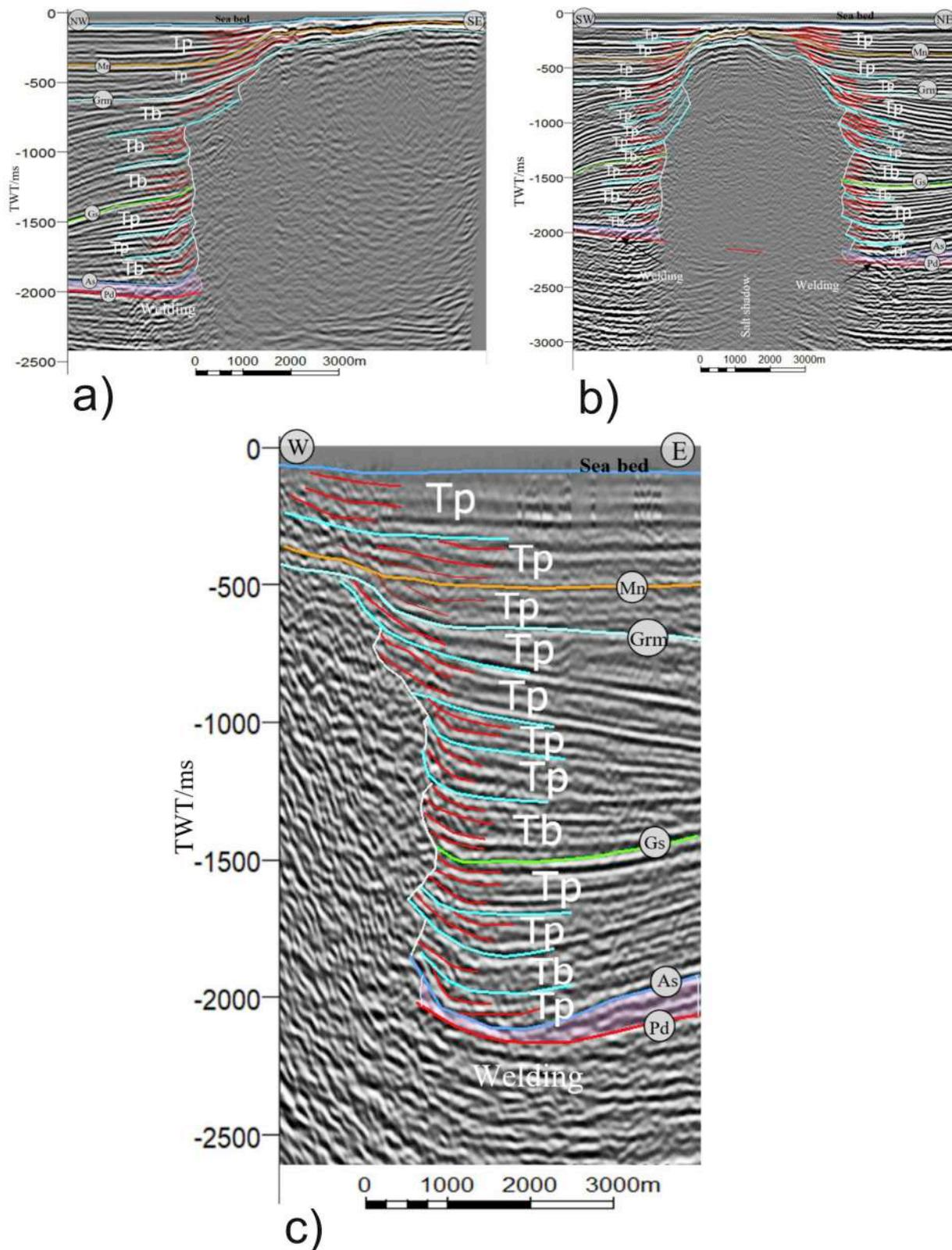
**Fig. 7.** (a–c) Interpreted seismic sections showing halokinetic sequences in the central salt structure, Abu Musa Diapir. Locations as per Figs. 4–6. “Tb” and “Tp” mark the tabular and tapered halokinetic sequences, respectively. Abbreviations in Fig. 2 caption. a) western flank of the central salt structure, b) northern flank of the central salt structure and c) eastern flank of the central salt structure.
