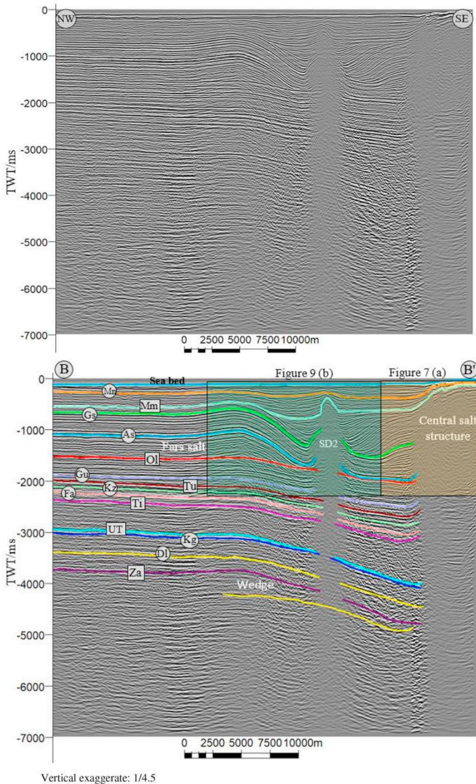
Fig. 5. Un-interpreted and interpreted BB' seismic sections NW-SE through the Abu Musa diapir. The interpreted SD2 and the central salt structures, the location of seismic horizons (letters in circles) and major unconformities (letters in rectangles) are shown. Abbreviations as per Fig. 2 caption. Locations of Figs. 7 and 8 shown by rectangles.
