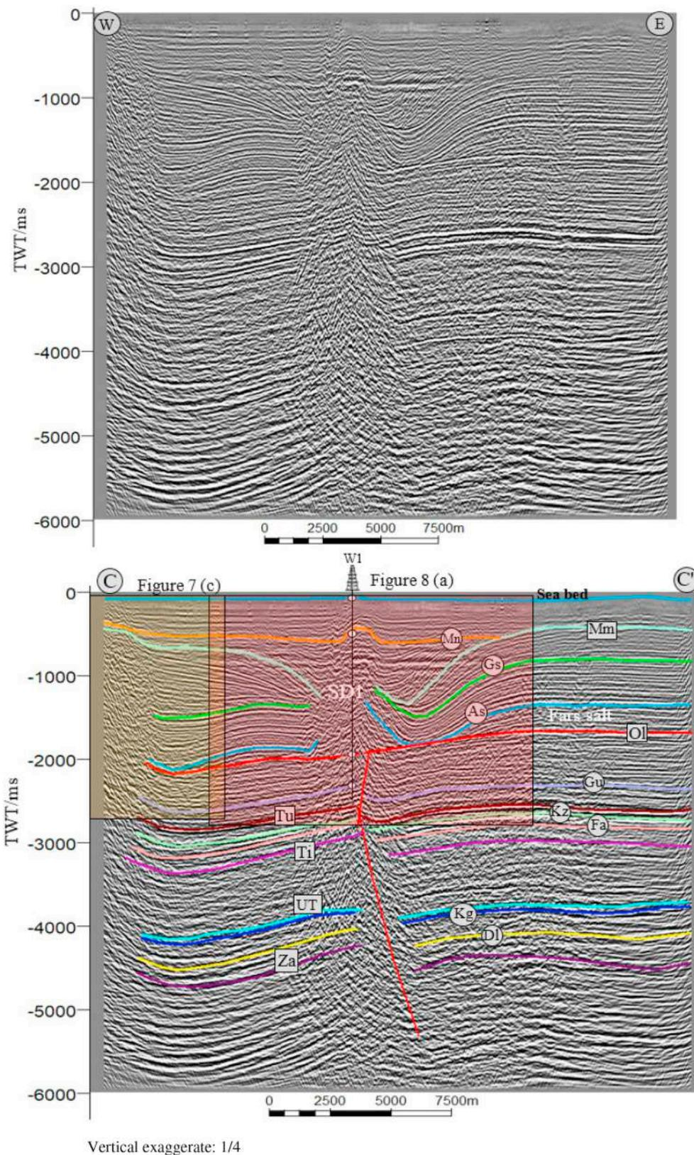
**Fig. 6.** Un-interpreted and interpreted CC' seismic sections E-W around the Abu Musa diapir. The interpreted SD1 and central salt structures and the location of seismic horizons (letters in circles) and major unconformities (letters in rectangles) are shown. Abbreviations as per Fig. 2 caption. Locations of Figs. 7 and 8 shown by rectangles.
