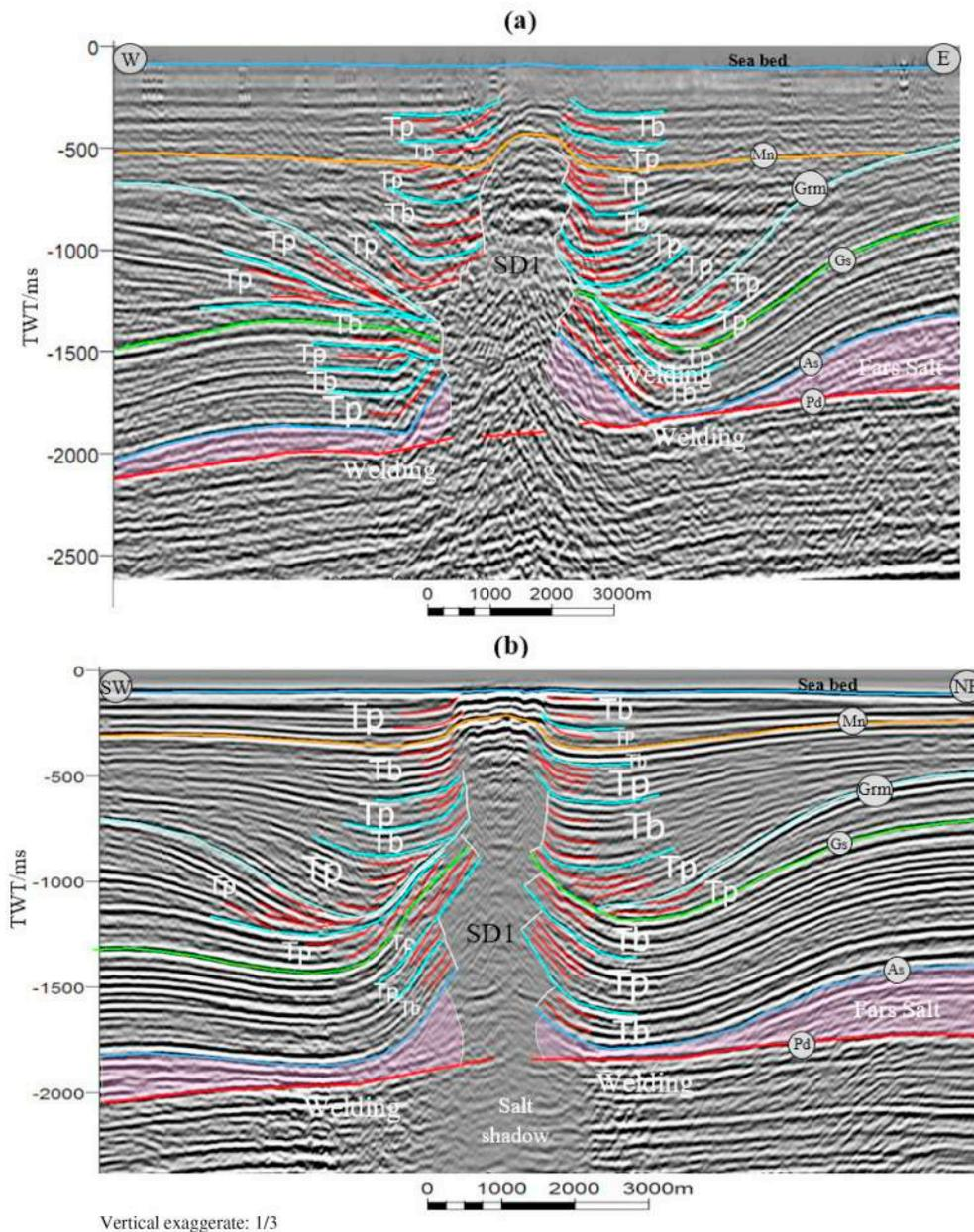
Fig. 8. (a, b) Un-interpreted and interpreted seismic sections showing halokinetic sequences on the SD1 salt structure along AA' and CC' (locations as per Figs. 4 and 6). "Tb" and "Tp" mark the tabular and tapered halokinetic sequences, respectively. Details of the used letters in Fig. 2.
