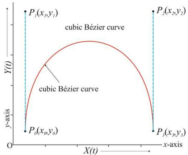
Fig. 1 An example of a cubic Bézier curve produced from plotting of  $X(t)$  and  $Y(t)$  (based on Eqs. 5 and 6) for  $t \in [0, 1]$  is an the control points  $P_0, P_1, P_2$  and  $P_3$  with coordinates  $(x_0, y_0), (x_1, y_1), (x_2, y_2)$  and  $(x_3, y_3)$ , respectively
