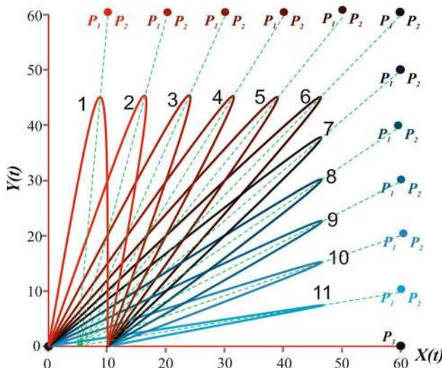
**Fig. 6** 11 different inclined isoclinal curves has been produced by keeping control points  $P_1$  and  $P_2$  as same point  $(x_a, y_a)$  which has been shifted from (10, 60) to (60, 60) and then from (60, 60) to (60, 10). It has been found that axial trace of each curve follows  $(x_a, y_a)$ .  $P_0$  and  $P_3$  has been kept fixed at (0, 0) and (10, 0), respectively, for the test
