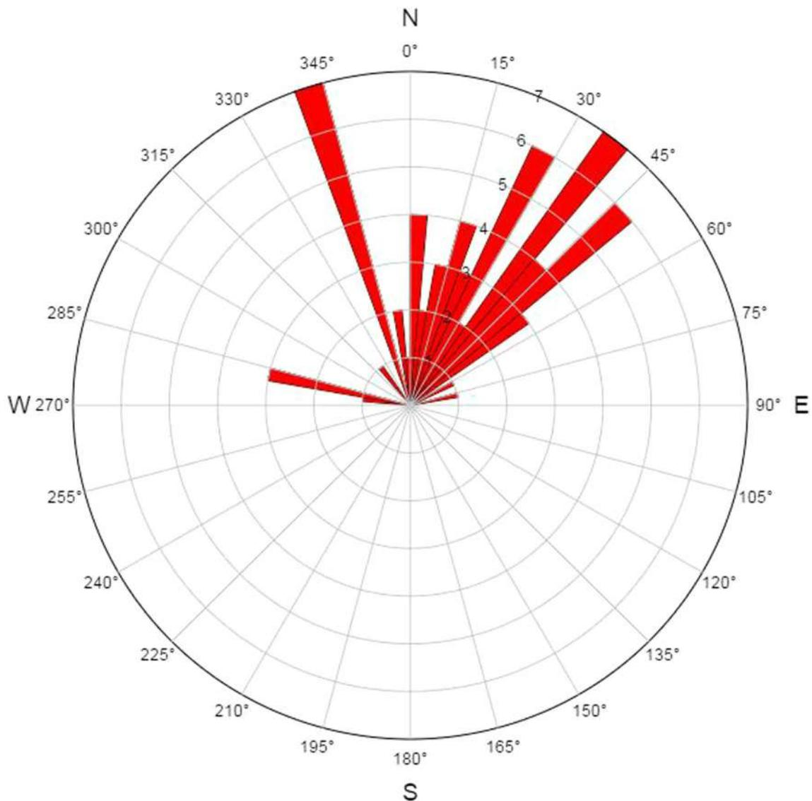
Fig. 13 Rose diagram shows the trends of strike-slip faults from the studied sections
