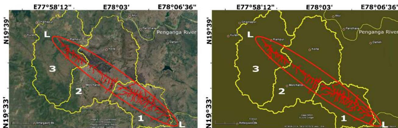
**Fig. 15** **a** Un-interpreted image showing Trellis drainage pattern (circled) along the Kinwat lineament shown on Google earth image, where 1–3: sub-basins, LL: Kinwat lineament. **b** Interpreted image showing trellis drainage. The main river is Penganga river
