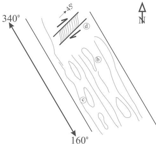
**Fig. 11** A schematic sub-horizontal exposure shows the position of the features in Figs. 10b–d. The zone trends 160°–340°. At position 'd', S- and C-fabric is well developed. C plane trends N45°E. 'b', 'c' and 'd' in circle indicate the line diagram of actual photographs of the structures shown as 'b', 'c' and 'd'
