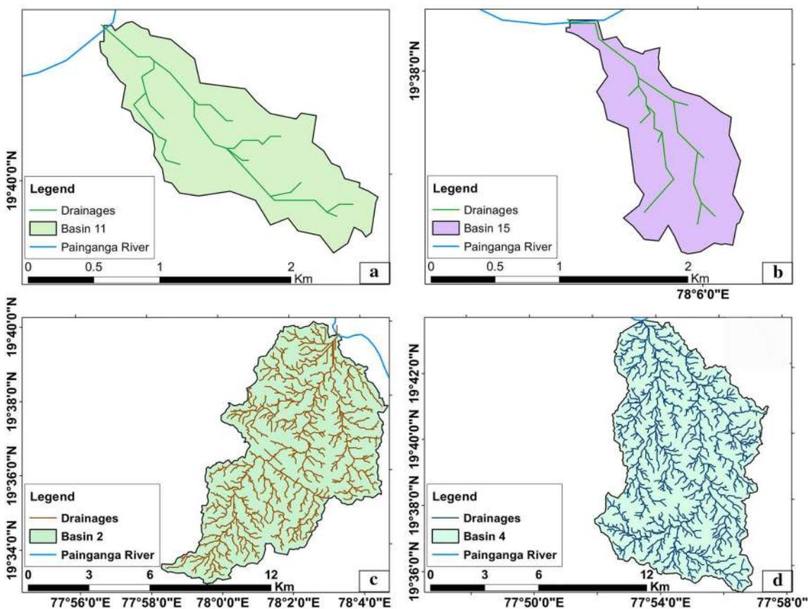
**Fig. 16** Represents development of dendritic drainage pattern with different number of streams i.e. **a** Sub-basin number 11 total number of streams 11, **b** sub-basin number 15 total number of streams 10, **c** sub-
