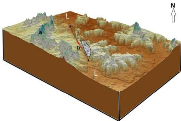
Fig. 14 Kinwat lineament exposed in the form of (a) hilly terrain in the bordered area of the basin and (b) deep valley in the centre. Black and red arrows in the centre indicate the directions of streams flowing along the lineament (L–L shown as white letters)
