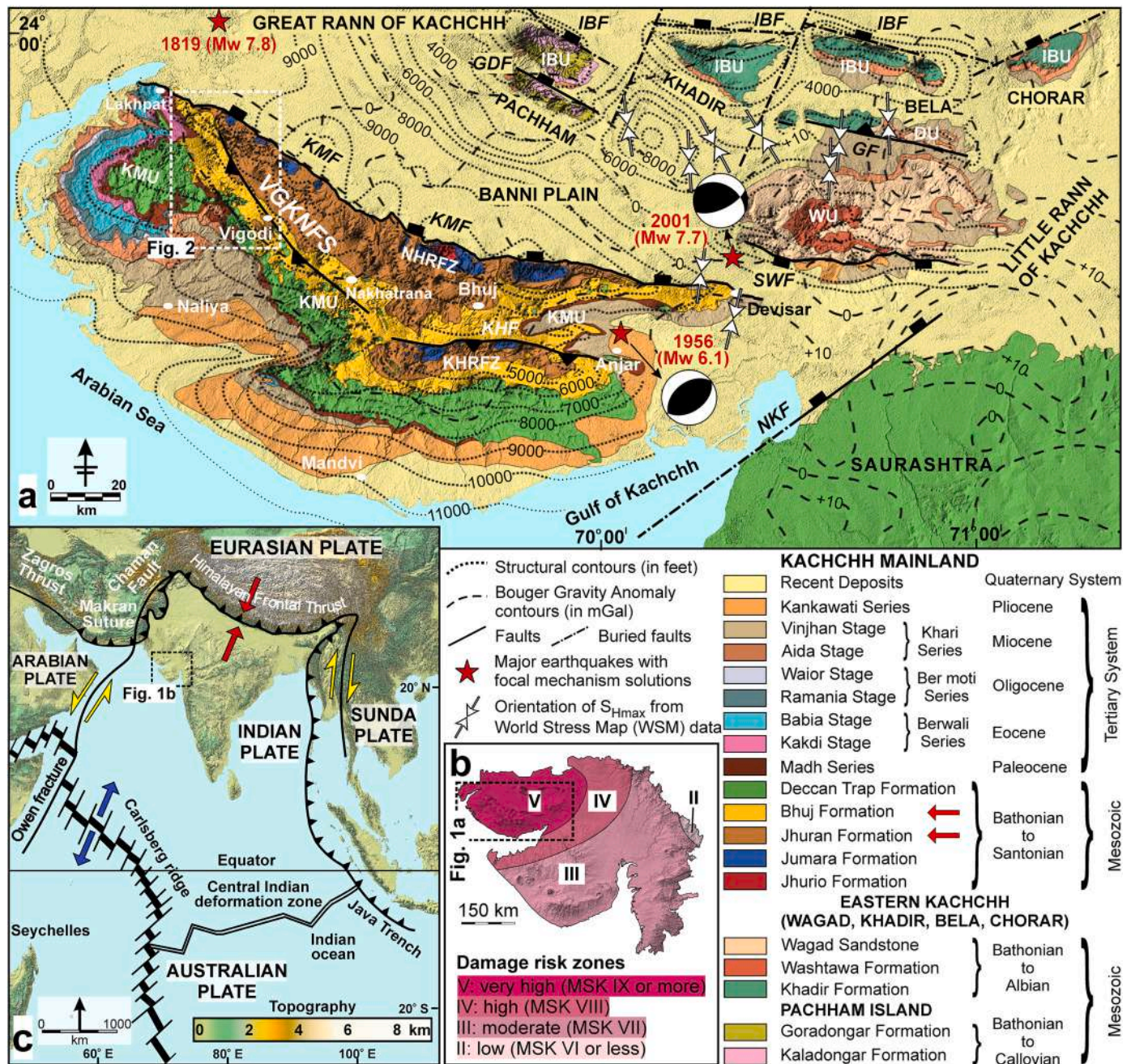
Fig. 1. (a) Geological map of the Kachchh Rift Basin (KRB), digitized and redrawn by Patidar (2010). Geological details are after Biswas (1993). The white inward-pointed double arrows represent the orientation of horizontal maximum compressive stress ( S_{Hmax} ) compiled from the World Stress Map (WSM) project (Heidbach et al., 2016, 2018). The black dotted lines represent structural contours with 1000 feet (values are in negative) contour interval drawn over the top of Precambrian basement (Biswas, 1993). The black dashed lines represent Bouguer Gravity Anomaly contours in mGal after Dasgupta et al., 2000. Red stars indicate major earthquakes in the KRB with focal mechanism solutions (Chung and Gao, 1995; Rastogi et al., 2001). IBF: Island Belt Fault, GDF: Gora Dungar Fault, GF: Gedi Fault, SWF: South Wagad Fault, KMF: Kachchh Mainland Fault, VGKNFS: Vigodi-Gugriana-Khirasra-Netra Fault System, KHF: Katrol Hill Fault, NKF: North Kathiawar Fault. IBU: Island Belt Uplift, DU: Desalpar Uplift, WU: Wagad Uplift, KMU: Kachchh Mainland Uplift, NHRFZ: Northern Hill Range Fault Zone, KHRFZ: Katrol Hill Range Fault Zone. Nature of the uplift-bounding faults is based on Biswas (1993); Patidar et al. (2007); Maurya et al. (2013), (2016), (2017). (b) Seismic hazard zonation map of Gujarat state after BIS (2002). Red, blue and yellow double arrows denote the direction of relative plate motion at convergent, divergent and transform-fault boundaries respectively. (c) Location of Gujarat state with respect to the Indian plate boundaries depicting various tectonic elements (redrawn after Chatterjee et al., 2013). Red, blue and yellow double arrows denote the direction of relative plate motion at convergent, divergent and transform-fault boundaries respectively.
