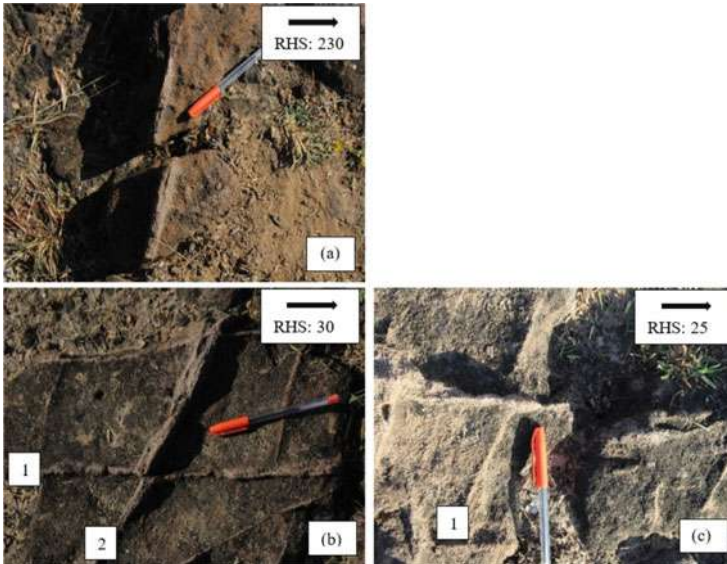
Fig. 9 Vein displaced/folded against or near another vein. Horizontal outcrop of sandstone along Kodhki Road. a Strike of vein-1: 160°. Dip: 80°. Dip direction: 70°. b Strike of vein-1: 160°. Dip: 85°. c Strike of vein-1: 25°. Dip: 70°
