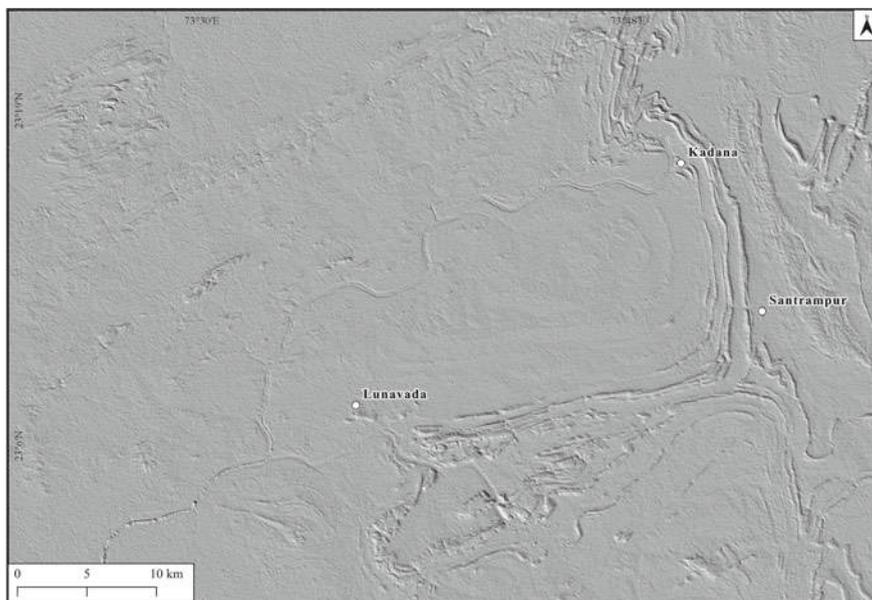
**Fig. 13** Hillshade derived from ASTER GDEM with azimuth of 225° and solar elevation of 45°
