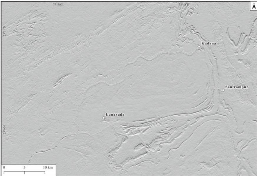
**Fig. 12** Hillshade derived from ASTER GDEM with azimuth of 180° and solar elevation of 45°
