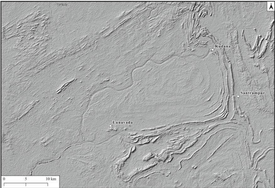
**Fig. 16** Merging of two hillshades with azimuth 315° and 45° and solar elevation of 45°
