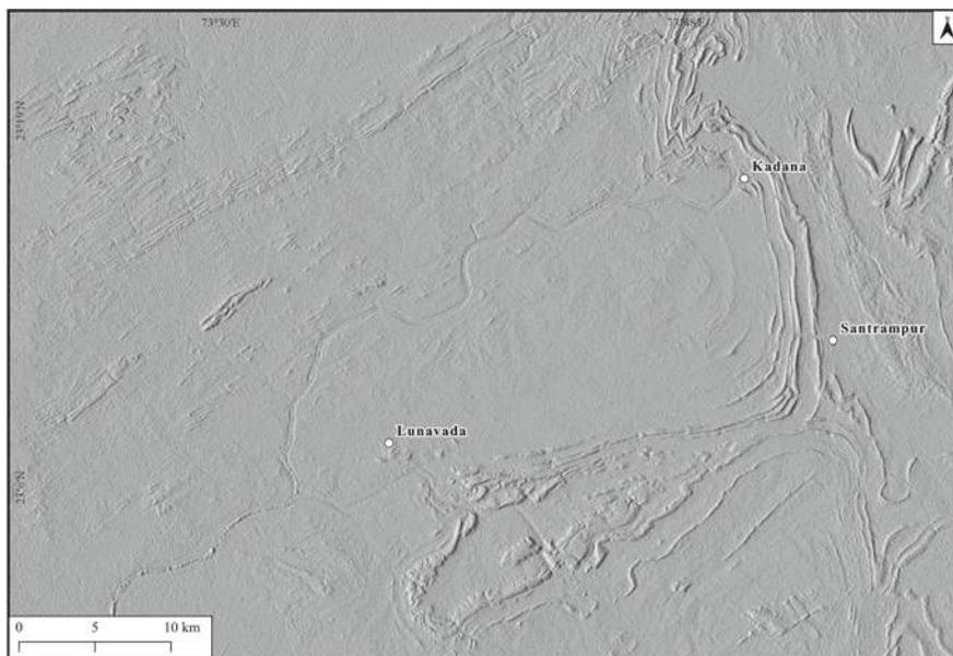
**Fig. 14** Hillshade derived from ASTER GDEM with azimuth of 270° and solar elevation of 45°
