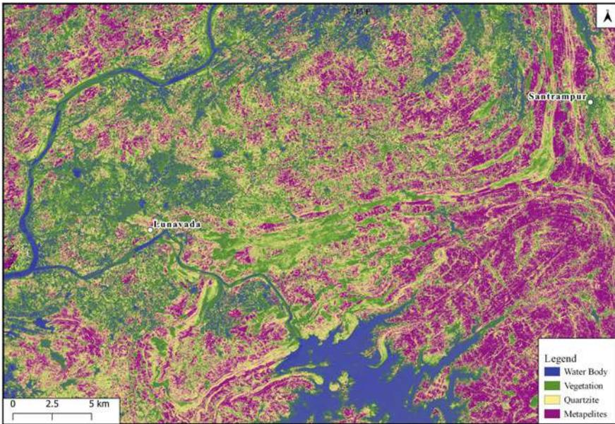
**Fig. 2** Sentinel-2 image displaying intercalation of quartzite with metapelites generated using band ratio of band 4(red) by band 2(blue) after applying ATCOR
