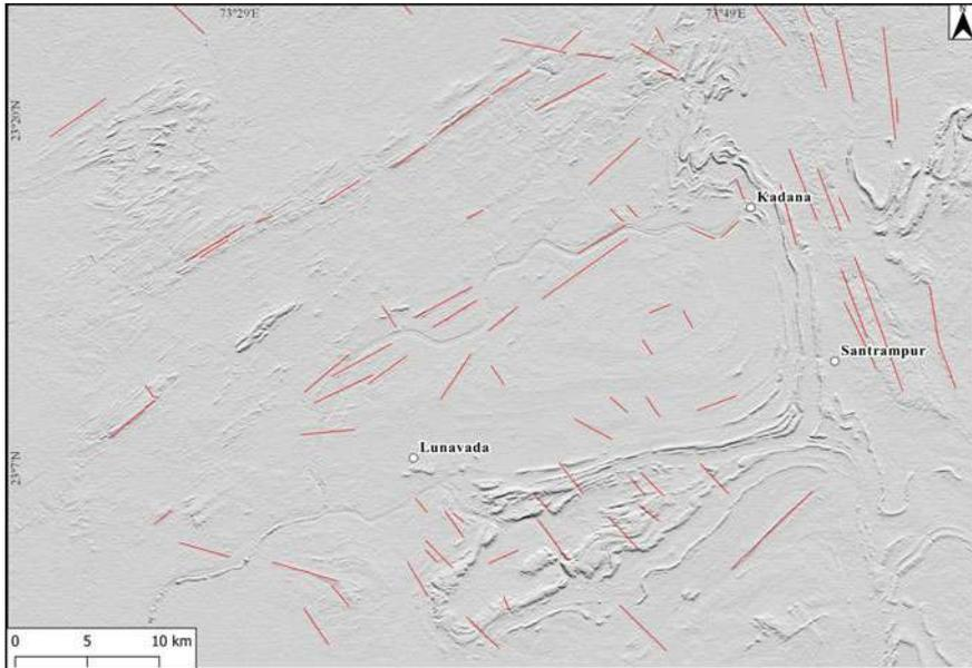
**Fig. 19** Lineaments extracted by merging two hillshades with azimuth of  $315^\circ$  and  $45^\circ$  and solar elevation of  $45^\circ$
