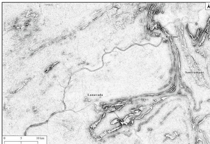
**Fig. 17** Positive openness map (enhancing surface upward)
