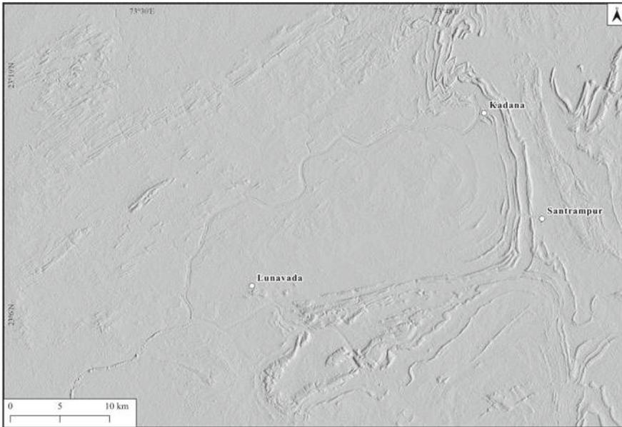
**Fig. 10** Hillshade derived from ASTER GDEM with azimuth of  $90^\circ$  and solar elevation of  $45^\circ$
