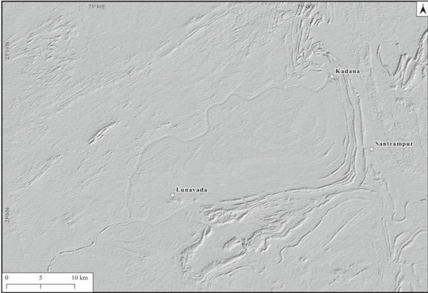
**Fig. 11** Hillshade derived from ASTER GDEM with azimuth of 135° and solar elevation of 45°
