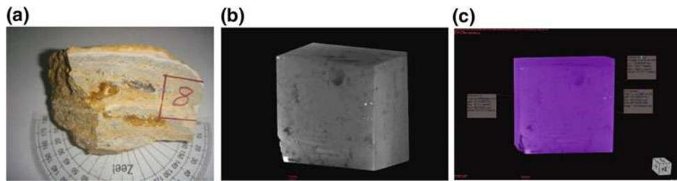
**Fig. 4** **a** Picture shows the sample 8, cut into 2 cm cube for XRCT scanning. **b** Sample 8 in three-dimensionality illustrate fabrics, pores, and overall structure. **c** XRCT image gives information about the pore
