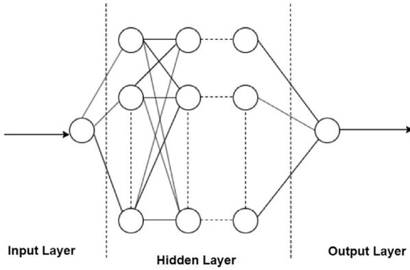
Fig. 4. A typical feedforward MLP neural network.
