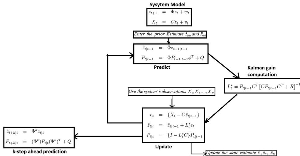
Fig. 2. Block diagram representing the estimation and forecasting by Kalman filter.
