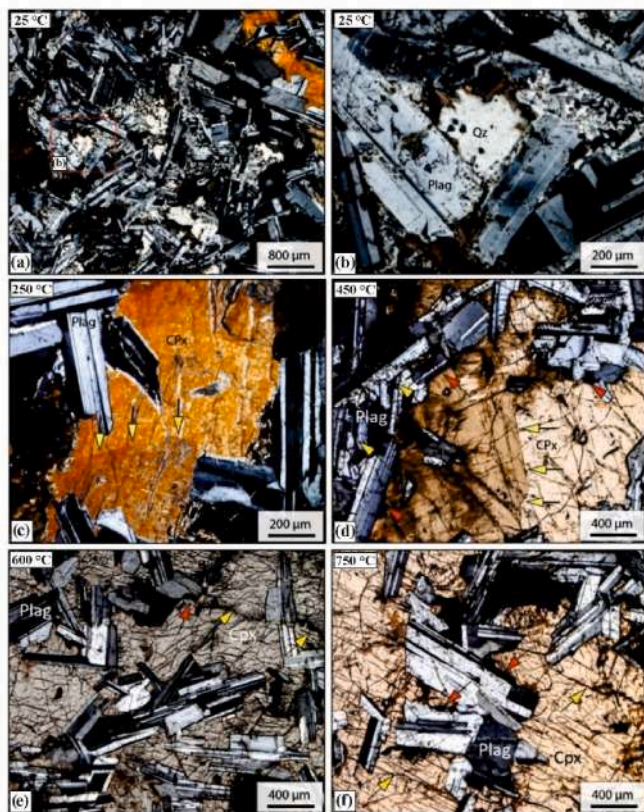
Fig. 2. Photomicrographs of dolerite samples treated at different experimental temperatures. The yellow arrows point to the intergranular fractures, and the red arrows to intragranular fractures (Plag: Plagioclase; Cpx: Clinopyroxene (Augite); Qz: Quartz).
