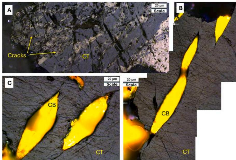
**Fig. 17.** (A) Isolated straight sub pattern cleat in collotelinite, (B) and (C) Partially isolated elliptical shape with pointed ends, cracks in collotelinite, filled with carbonates, Location: Near Dumerbera Village, West Bokaro basin.
