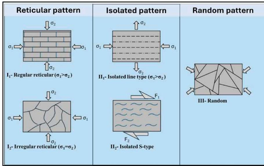
Fig. 3. The cleat network patterns include I<sub>1</sub>, regular reticular; I<sub>2</sub>, irregular reticular; II<sub>1</sub>, isolated straight; II<sub>2</sub>, isolated S-shaped; and III, random pattern. Here  $\sigma_1$  and  $\sigma_2$  indicate the maximum and the minimum principal stresses, respectively, and F denotes the shear force. After (Su et al., 2001).
