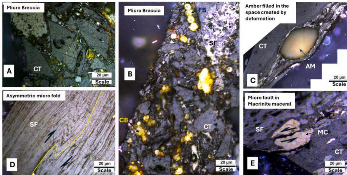
**Fig. 19.** (A) and (B) Micro coal breccia, (C) Amber filled by space created after deformation, (D) Asymmetric micro-fold, Micro fault in macrinite maceral (MC) Location: Near Dumerbera Village, West Bokaro basin. (CT- Collogerlinite, SF- Semifusinite, FB- Framboidal Pyrite, Am- Amber, CB- Carbonate).
