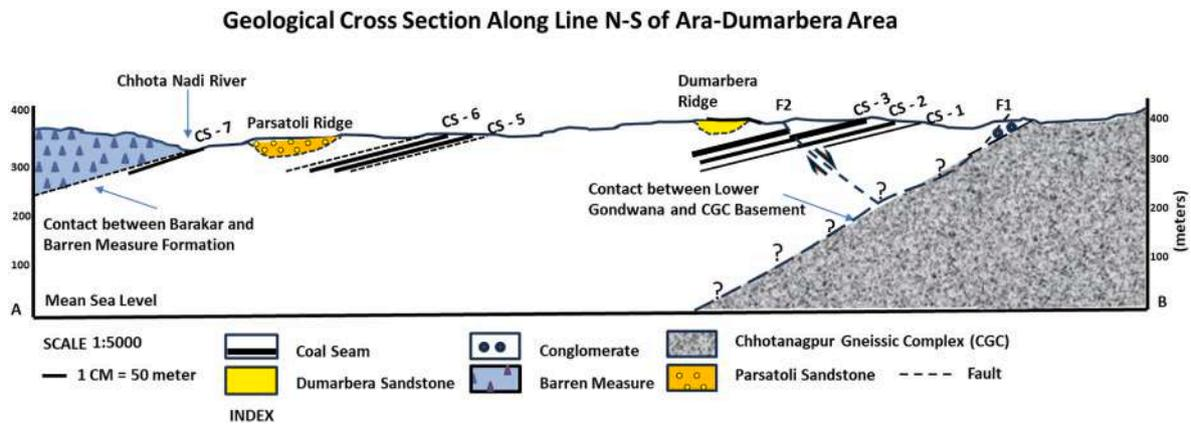
Fig. 11. Geologic cross-section prepared along the traverse A and B shown in the map (Fig. 7), the traverse starts at the southern margin of the West Bokaro basin across the CGC, Barakar Formation and Barren Measures.
