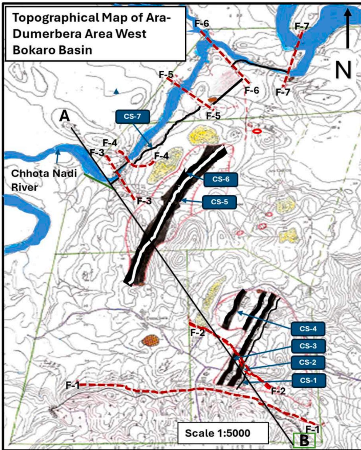
Fig. 7. Topo-map of the study area, Location: Ara-Dumerbera village, West Bokaro basin, A-B Traverse taken for the preparation of geological cross section, CS- Coal Seam (Black Colour), F- Fault (dashed red line).
