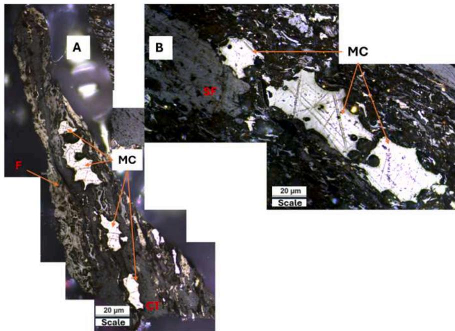
**Fig. 20.** Boudinage like structure Location: Near Dumerbera Village, West Bokaro basin. (MC- Macrinite, SF- Semifusinite, F- Fusinite, CT- Collotelinite).
