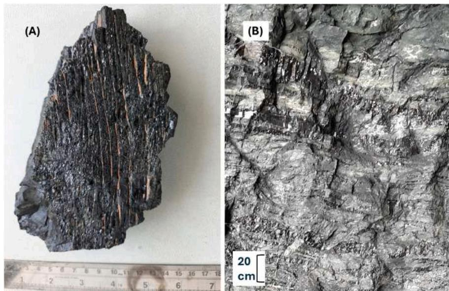
**Fig. 8.** (A) I, regular reticular cleat, the development is attributed to the compression, as per [Su et al. \(2001\)](#), the cracks are filled by secondary clay minerals (B) a fresh cut section of Seam 6 from the Ara-Dumerbera area of the West Bokaro basin, where coal is marked by the bright and dull bands. Development of multiple set of cleats within the bright band are particularly noticeable and may be classified as gas expanding fractures/cleats.
