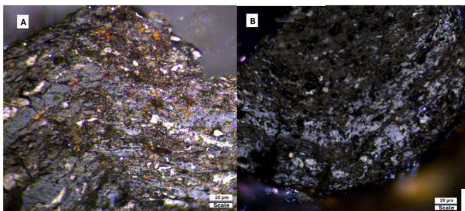
Fig. 21. Fold appeared in partially crushed, amalgamated coal macerals, Location: (A) East Bokaro Basin and (B) West Bokaro Basin.
