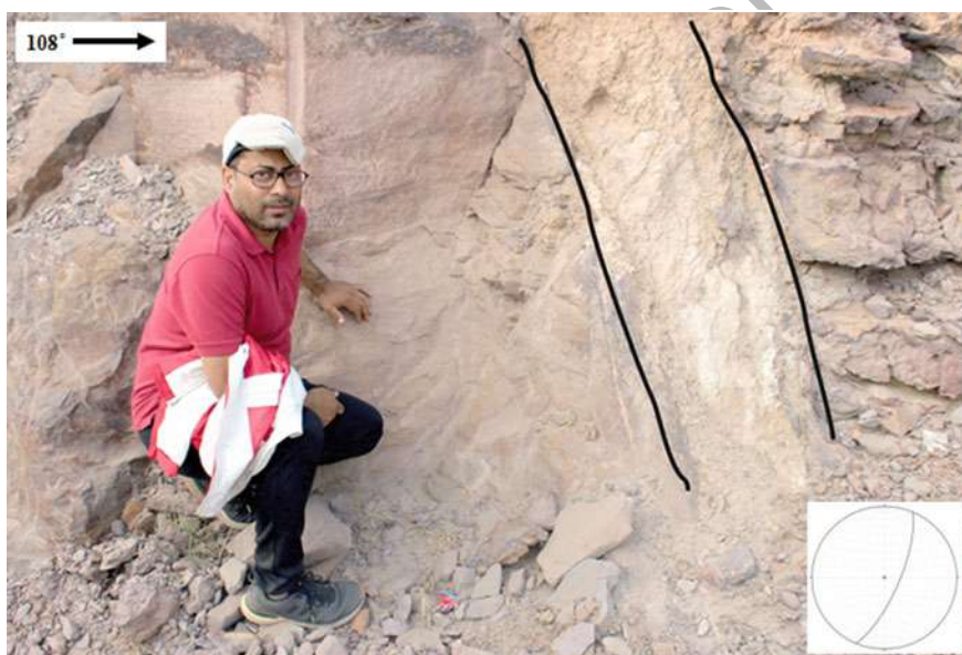
Fig. 18 Vertical section of a thick white colored fault gouge (attitude: dip amount 70^{\circ} , dip direction 113^{\circ} , strike 23^{\circ} ) in Early Cretaceous sandstone of Lower Bhuj succession. Soumyajit Mukherjee (174 cm) is shown as scale. Location: Kodki road fault, near Bhuj city, Gujarat, India. 23^{\circ} 14' 38.228'' N, 69^{\circ} 35' 8.286'' E
