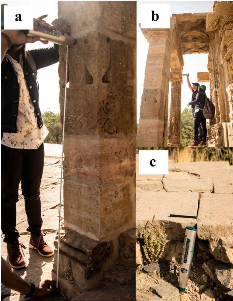
Fig. 29 Strength measurement with Smith Hammer at the pillars of the Shiva Temple (Temple no. 4) in a vertical direction, b horizontal direction, c Basalt base of Jagati (Smith hammer marker of length 24 cm)
