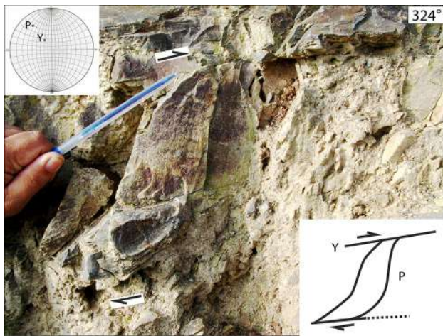
Fig. 4 Top-up-to-the-NW brittle shear, within Rautgara Slate, Inner Lesser Himalaya, is defined by sigmoid-shaped P -plane, bound by two sub-parallel Y -planes. Inset stereo-plots of poles of Y - and P -planes. The inset line traces the right margin of the sigmoid
