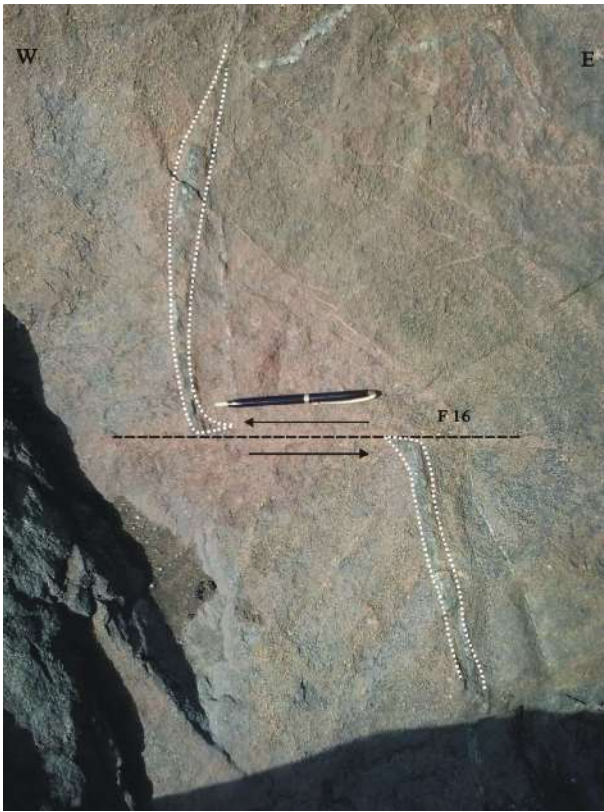
Figure 6. Brittle-ductile sinistral shear on the E striking fault plane. Observed on a near horizontal plane. At site 1, Gokunda; see figure 1 for location. Length of pen: 14 cm.
