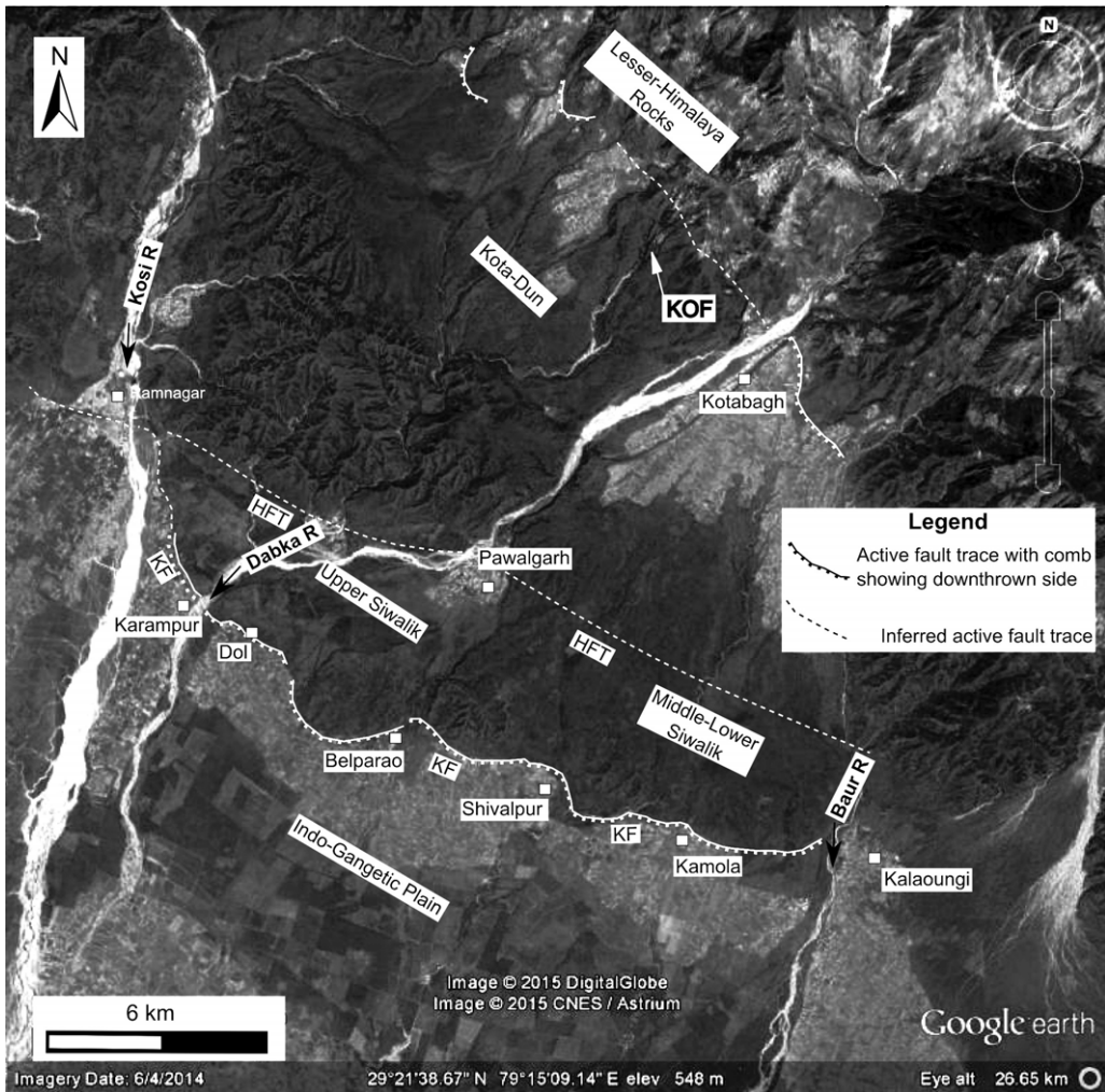
Fig. 8. Out-of-sequence thrusts around Kaladungi–Kotabagh area (Nainital). Quickbird image with 2.4 m resolution in the RGB bands. Source: http://www.satimagingcorp.com/satellite-sensors/quickbird/ (last accessed on 25 February 2015) This figure was prepared independently, following Malik et al. (2014, fig. 1), by Achyuta Ayan Misra (Indian Institute of Technology Bombay). KOF, Kotabagh Fault; KF, Kaladungi Fault; HFT, Himalayan Frontal Thrust.
