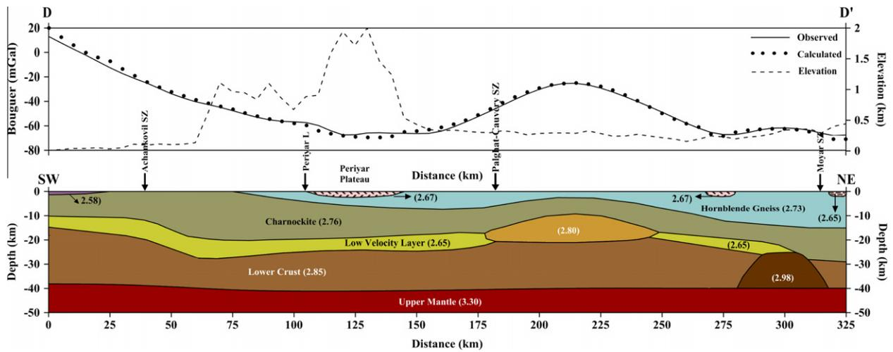
Fig. 11. Gravity derived crustal model along profile DD'. The values represent densities in  $\text{g}/\text{cm}^3$ . SZ: shear zone; L: lineament.
