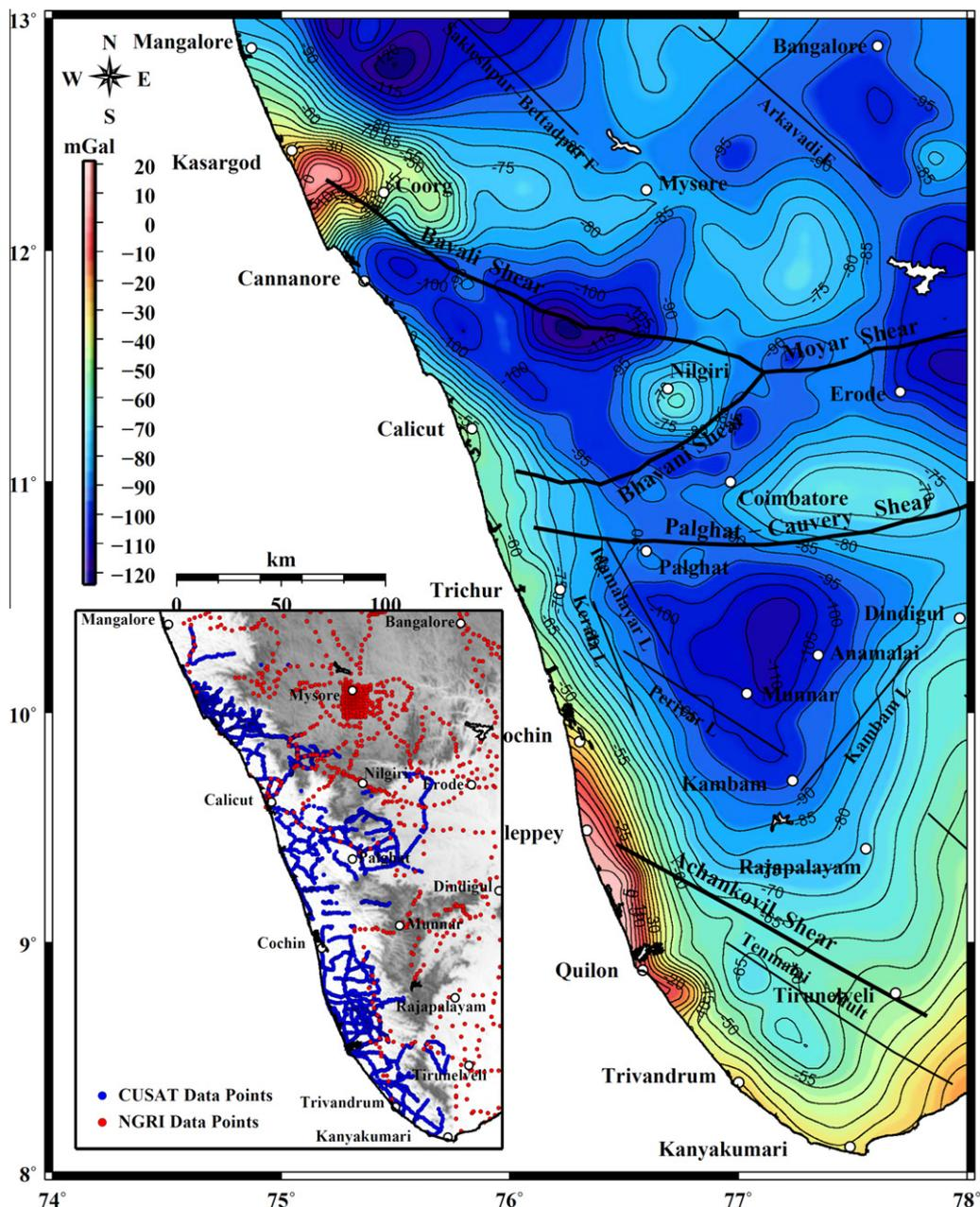
Fig. 3. Bouguer anomaly map of south western part of SGT prepared at 5 mGal contour interval. Shear zones, lineaments (L) and faults (F) are shown for comparison. The inset represents the distribution of gravity data points in the area.
