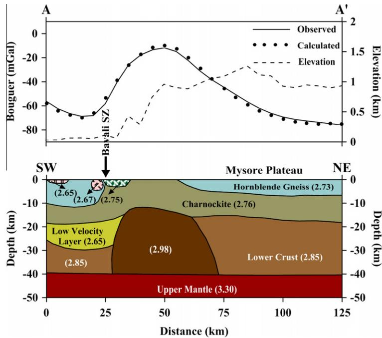
Fig. 8. Gravity derived crustal model along profile AA'. The values represent densities in  $\text{g}/\text{cm}^3$ . SZ: shear zone; L: lineament.
