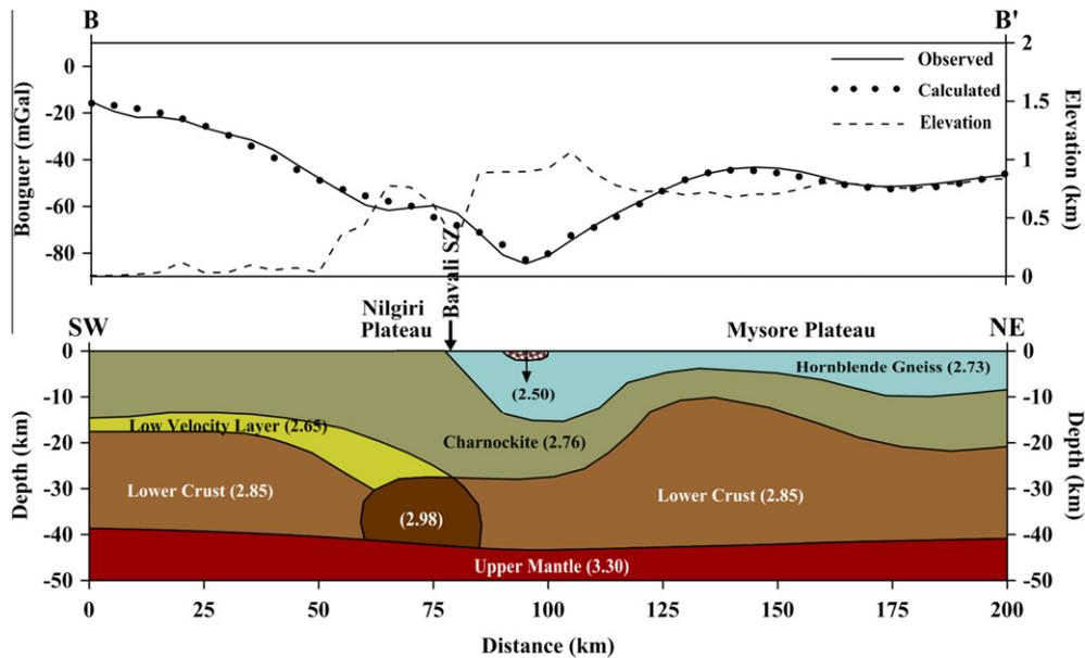
Fig. 9. Gravity derived crustal model along profile BB'. The values represent densities in  $\text{g}/\text{cm}^3$ . SZ: shear zone; L: lineament.
