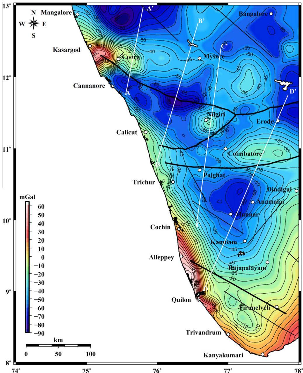
Fig. 5. Geoidal Corrected Bouguer Anomaly (GCBA) map of the study area. Contour interval 5 mGal. Lines AA' through DD' represents profiles selected for two-dimensional gravity modeling.
