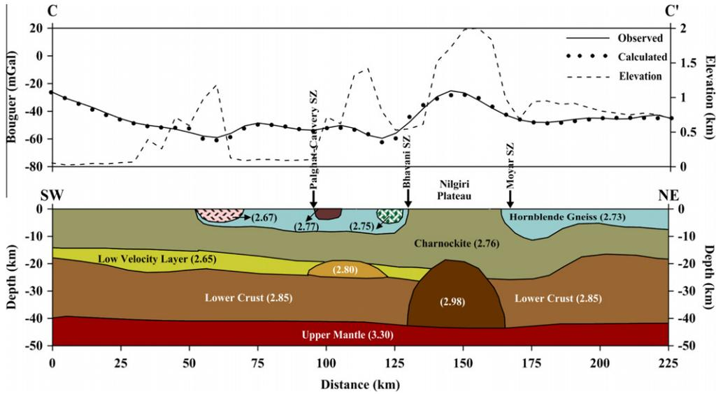
Fig. 10. Gravity derived crustal model along profile CC'. The values represent densities in  $\text{g}/\text{cm}^3$ . SZ: shear zone; L: lineament.
