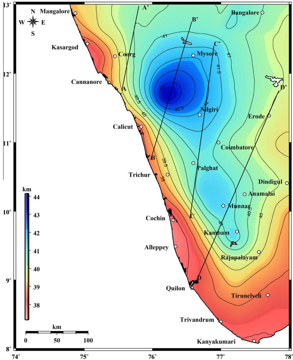
**Fig. 7.** Crustal thickness map for fully compensated regional topography assuming 38 km as standard crustal column thickness at sea level, 0.4 g/cc as density contrast of crust with mantle and density of regional topographic mass as 2.75 g/cm<sup>3</sup>. The contours represent the Moho depth in km. Lines AA' through DD' represents profiles selected for two-dimensional gravity modeling.
