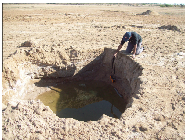
Fig. 4. Field photo of calcrete profile with anomalous \gamma -activity.
